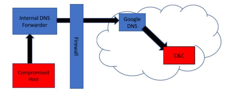
Figure 1: Illustrates a typical network Firewall with data being exfiltrated via DNS Traffic
